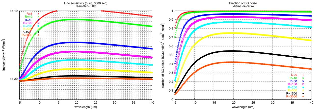
Figure 11. (left) Line Sensitivity of MIRACLE spectroscopy. Calculation is based on narrow band imaging case. In case of slit-spectroscopy, the sensitivity is slightly worse. Results of medium resolution spectroscopy are just for reference.
