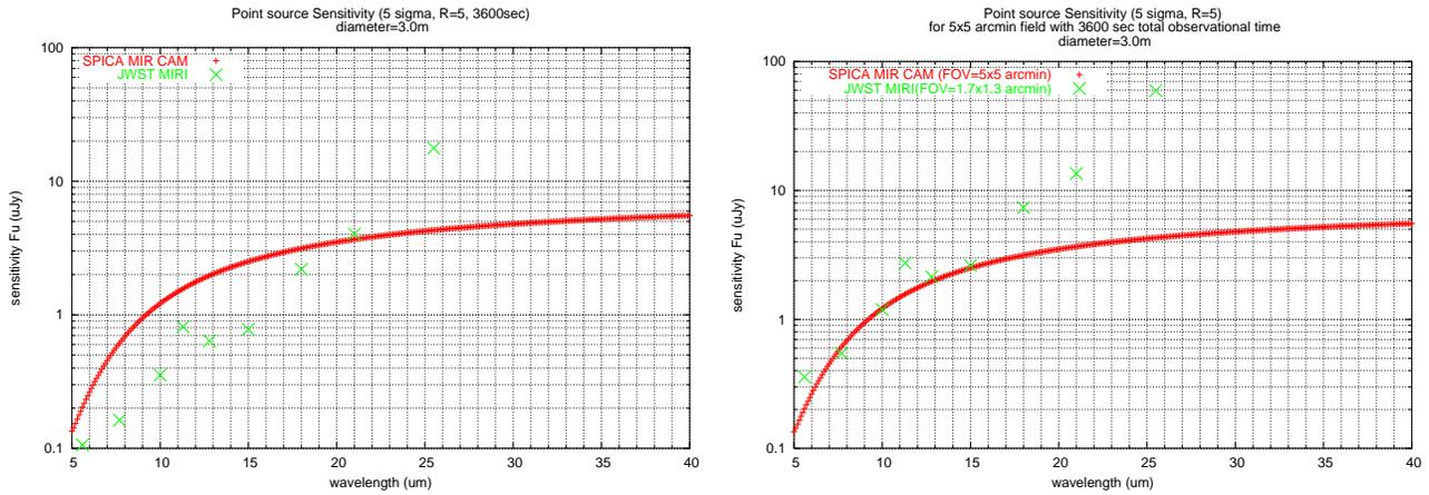
Figure 9. (left) Sensitivity of MIRACLE. Red plus signs show point source sensitivity ( $5\sigma$ ) of MIRACLE with one hour observing time in the imaging observations (spectral resolution  $R=5$ ) as a function of wavelengths. Green crosses show point source sensitivity of JWST/MIRI with the same integration. MIRACLE has superior sensitivity compared with JWST/MIRI over wavelengths of  $20\mu\text{m}$  because of SPICA's cooled aperture telescope.
