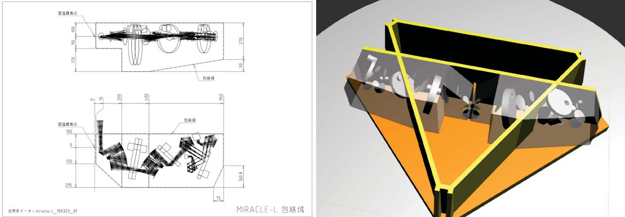
Figure 7. (left) Result of raytrace and Physical configuration of each optical and mechanical elements in MIRACLE-L. Both length and height are within system requirement size (1000mm and 400mm).
