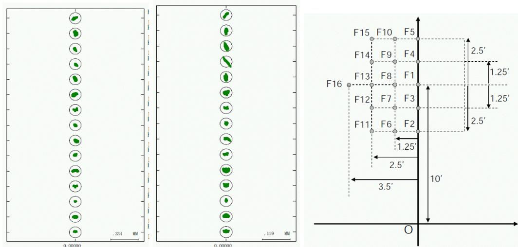
Figure 4. Spot diagram of MIRACLE-S and -L optics. The circles show the size of airy disc at the wavelength of  $5\mu\text{m}$ . The top spot diagram shows that at the position of F1 and the bottom shows that of F15.
