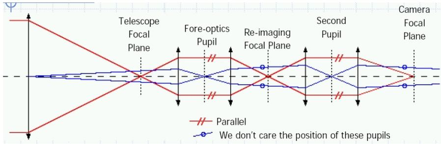
Figure 3. Design concept of MIRACLE optics.<sup>10</sup> A filter wheel is installed at the fore-optics pupil. A slit wheel is installed at the focus of fore-optics in order to impliment both wide field imaging and slit spectroscopy. A grating/mirror wheel is installed at the rear-optics pupil.
