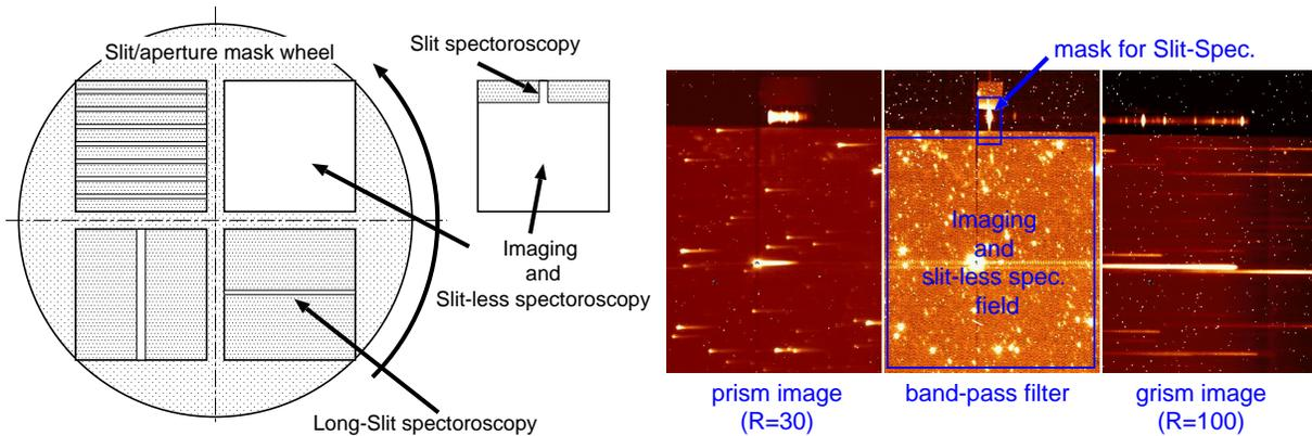
Figure 5. (left) Schematic of field mask/slit wheel.
