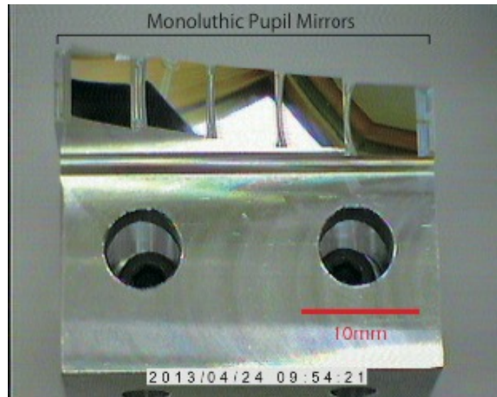
Figure 6. – The test piece of monolithic pupil mirrors for MRS-S produced using Nanoform 250 at Crystal Optics Ltd.
