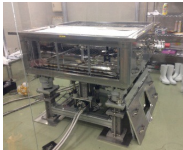
Figure 12. Cryogenic chamber for TTM mechanism test [12].
